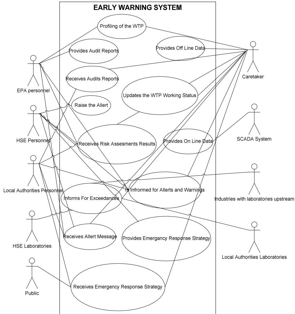
Fig. 1. UML Use Case Diagram depicting functional requirements as desired features of the early warning system
